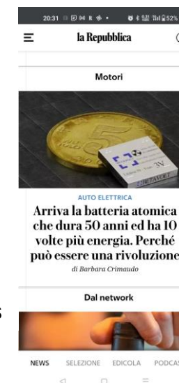
Betavolt-100 microwatts at 3V, 15x15x5 cubic millimeters
